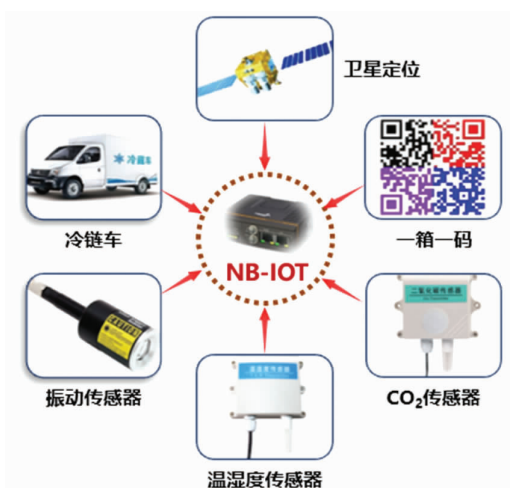
Fig.1 Integrated information acquisition system concerning about field detection and supply chain information of prefabricated food
